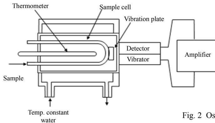
Fig. 2 Oscillator-type density meter
